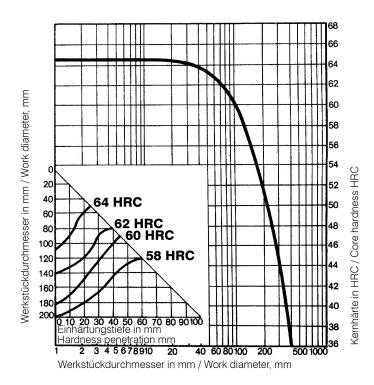
Hardening temperature: 950 °C (1742 °F) Quenchant: Oil
