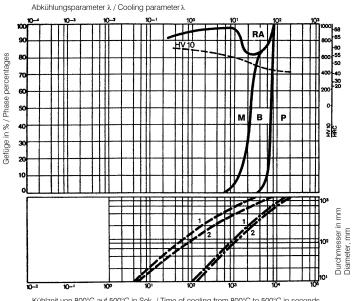
HV10... Vickers Hardness RA... Residual austenite M... Martensite B... Bainite
