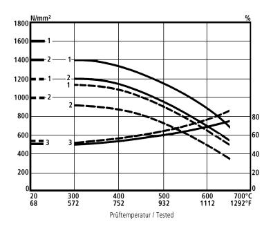
heat treated 1600 N/mm<sup>2</sup> heat treated 1200 N/mm<sup>2</sup> ... Tensile strength N/mm<sup>2</sup> 2... 0.2% proof stress N/mm<sup>2</sup>
