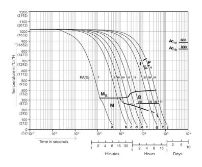
Austenitising temperature: 1020°C (1868°F) Holding time: 15 minutes 5...100 phase percentages 0.5...180 cooling parameter, i.e. duration of cooling from 800 - 500°C (1472-932°F) in s x  $10^{-2}$
