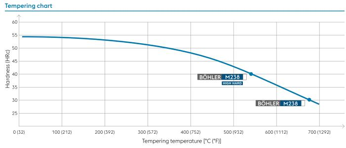
Hardening temperature: 850 °C (1562 °F) Specimen size: square 50 mm (1.97 inch)
